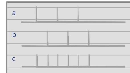
Two laser output combined with an adjustable delay to double the repetition rate of the pulse.
