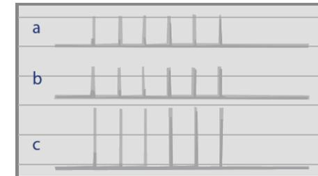
Two laser output synchronized to double the pulse energy and peak power,
