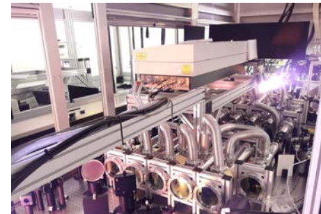
Intrepid HE: Intrepid I as a seeder on the top of and up to 6 PAMDAM on the table.
