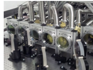
Image relay telescopes: high level of standardization
